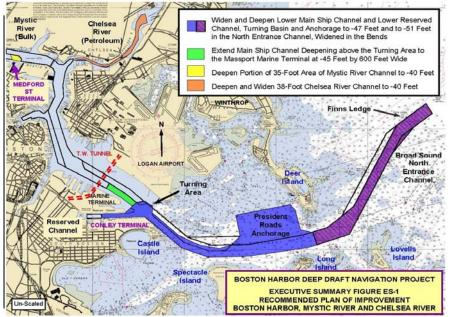
MLLW, -51 MLLW in the Broad Sound North Entrance Channel area. Massport, as the local sponsor for the Boston Harbor Deep Draft Navigational Project, also committed to construct two deep-water berths at Conley Terminal to a depth of -50 MLLW (three feet below the dredge depth of the Federal Channel). To
