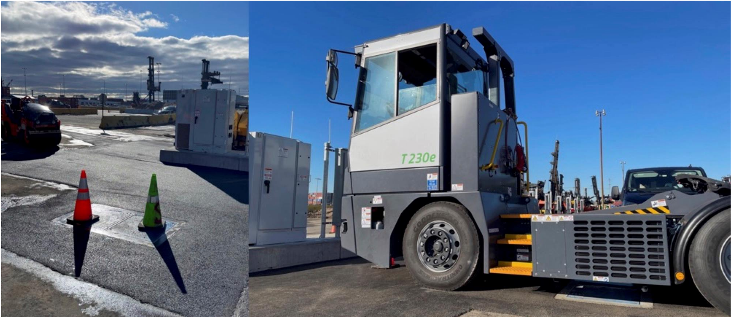
Seven (7) MAFI T230e yard tractors deployed with InductEV wireless charging in Port Elizabeth, New Jersey
